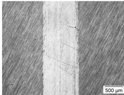
*Figure 4.5. Image of abrasion traces and uncoated SKD11 samples*
