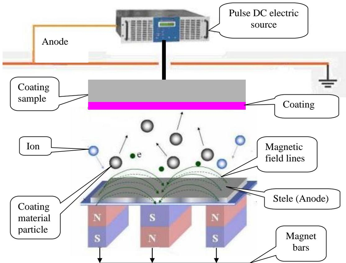
Figure 2.1. Operation principle of of the pulsed DC sputtering system
