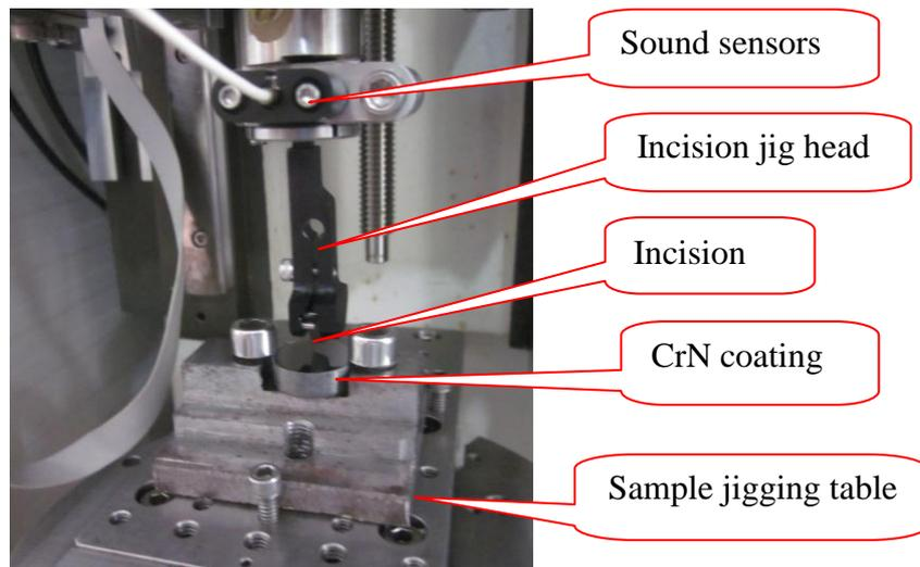
Figure 4.1. Adhesion measurement diagram of the CrN coating to SKD11 steel substrate on equipment UMT-2
