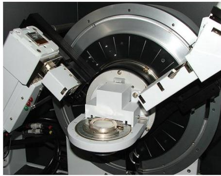
*Figure 3.3. X-ray diffraction measurement system (XRD)*
