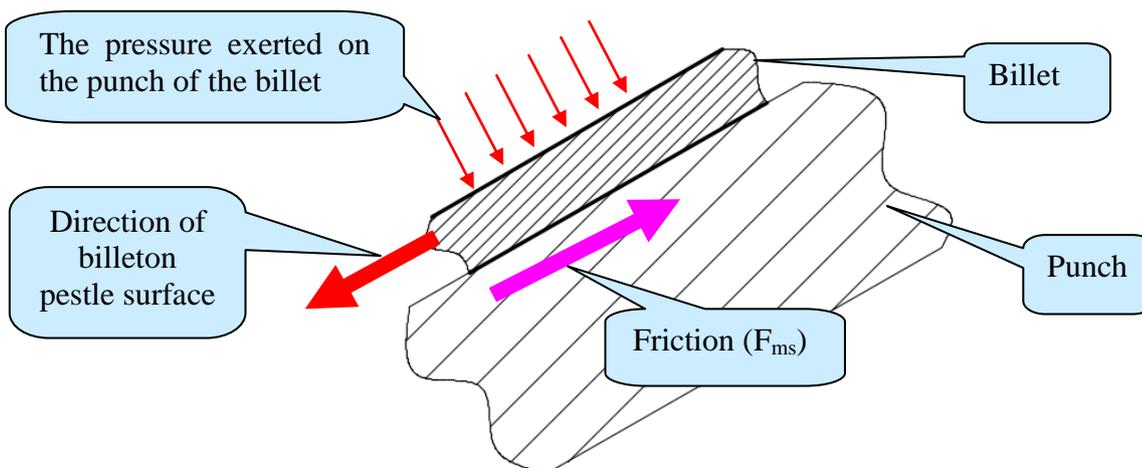
Figure 4.9. The slide of billet on the surface of the punch
