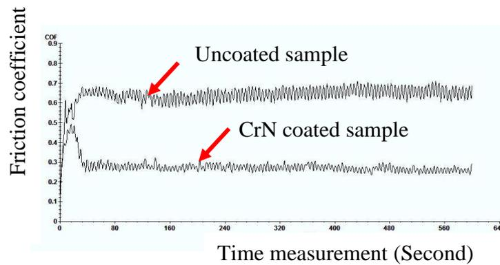
Figure 4.4. Representative friction coefficient of sample CrN coated and CrN uncoated over time
