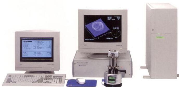
*Figure 3.4. Atomic force microscopy DI 300*
