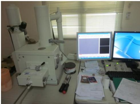
*Figure 3.2. scanning electron microscope (SEM/EDX) Jeol JMS 6490*
