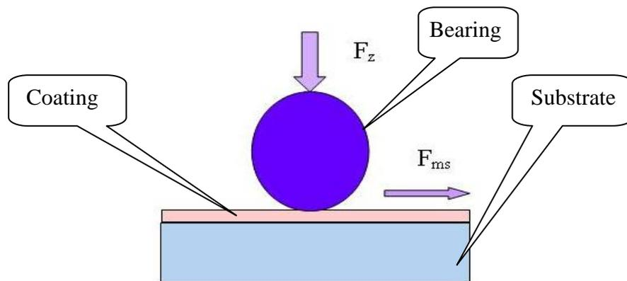
Figure 3.8. Measurement principle of friction and abrasion in form of reciprocating translation, bearing on flat samples
