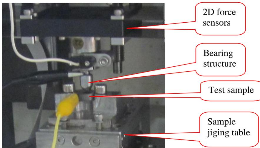
Figure 4.3. Friction measurement diagram and abrasion on equipment UMT-2
