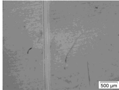
*Figure 4.6. Photo of abrasion traces of CrN coated SKD11 steel sample*
