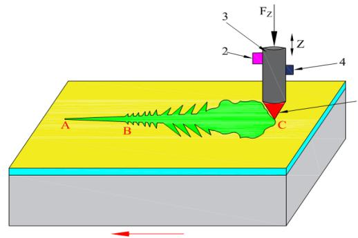
Figure 3.7. Principle of measuring the adhesion of the coating to the substrate
